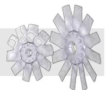
The **Flowtech**-propellers, hubs and blades are made of cast aluminum alloy, the aero-dynamical profile guarantees high efficiency and low noise. The blades are with adjustable pitch angle to optimum the duty point. The solidity varies for a wider range of performance. All rotating aluminum components are X-ray examined to ensure quality and reliability. All propellers are statically and dynamically balanced to ISO 1940 and AMCA 204 balance quality grade level-G2.5.
