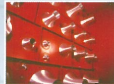
Multiple Nozzles for Flow Measurement
