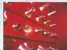
流量噴嘴 Multiple Nozzles for Flow Measurement
